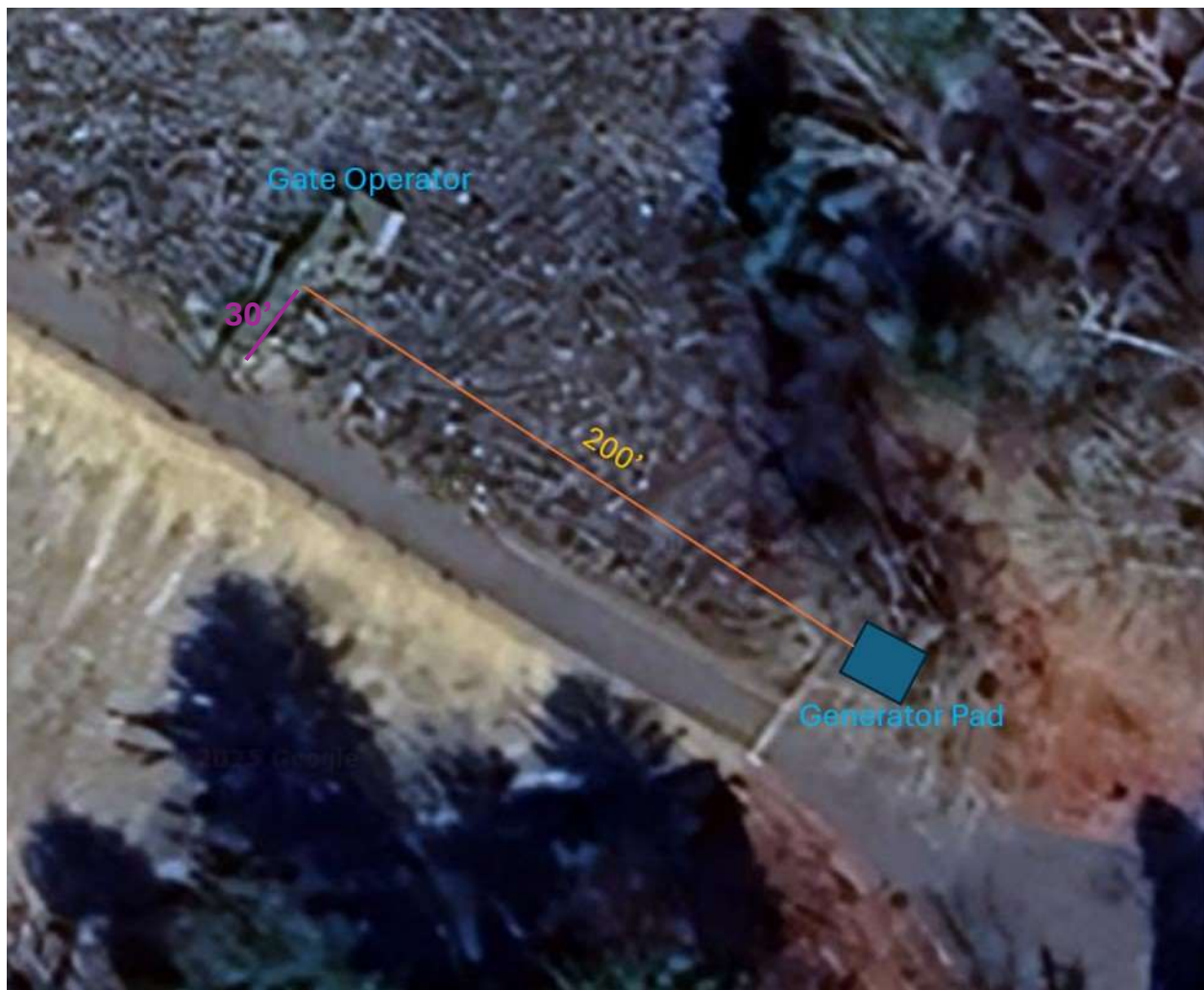
Image 2: Aerial photo showing conduit span to gate operator stairs/ pull box. Pull box at stairs has surface mounted 30' of 2" PVC conduit extending to the wood control panel.
